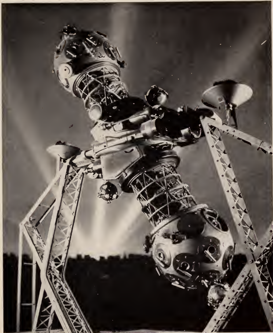
The Zeiss Projector of the Planetarium
