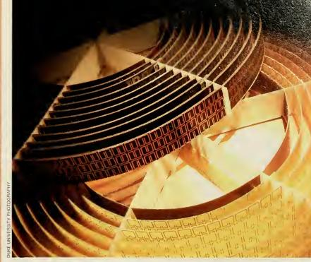
Two versions of a cloaking device created by Duke University engineers, using metamaterials, that makes invisibility possible at microwave frequencies. Each is one centimeter high and about ten inches across. Tiny electric circuits embedded in their concentric rings bend the path of microwave radiation in such a way that the electromagnetic waves flow around the cloaking device, making both it and an object placed in the center undetectable.
