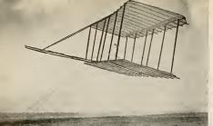
↑ The Wright's tethered glider at Kitty Hawk October, 1900. For lack of suitable winds, it was flown unmanned. Balancing was controlled from the ground by cords.
