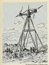
Sketch of a giant twinwheeled wind turbine to produce 6,500 kilowatts. Such a machine is possible but costs are prohibitive.
