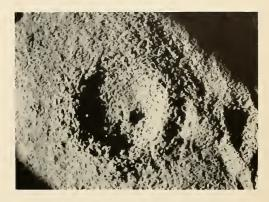
The central cone characteristic of many moon craters was produced accidentally in the laboratory when a very thin cement-dust surface was used. The central cone was discovered to be ground material not carried away from the center when the meteor struck and scattered
