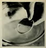
The model was then dipped repeatedly in liquid clay, to thoroughly cover all the fine structures.
