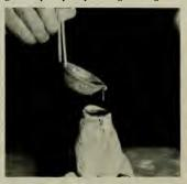
Molten gold was poured into the funnel opening to fill the space left by the "lost" wax model.
