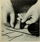
For casting an object such as this ear ornament, a model was made by assembling prepared wax threads.
