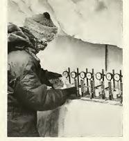
Long corers rest on a table in laboratory of snow mine. Short cores are kept on wall shelf.
