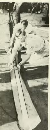
PULLING PIPE back over rod extrudes core onto wrapper on deck of the Vema.
