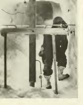
STRAIN GALGES measure distortion ice pressure causes in the walls of a South Pole ice tunnel.
