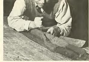
In Lamont Laboratory, the deep-sea core is split lengthwise and prepared
