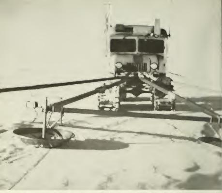
ELECTRONIC CREVASSE-DETECTORS on long beams are pushed ahead of a Sno-cat, above. Temporary station, below, near the center of Ross Ice Shelf, was site of three-day series of
