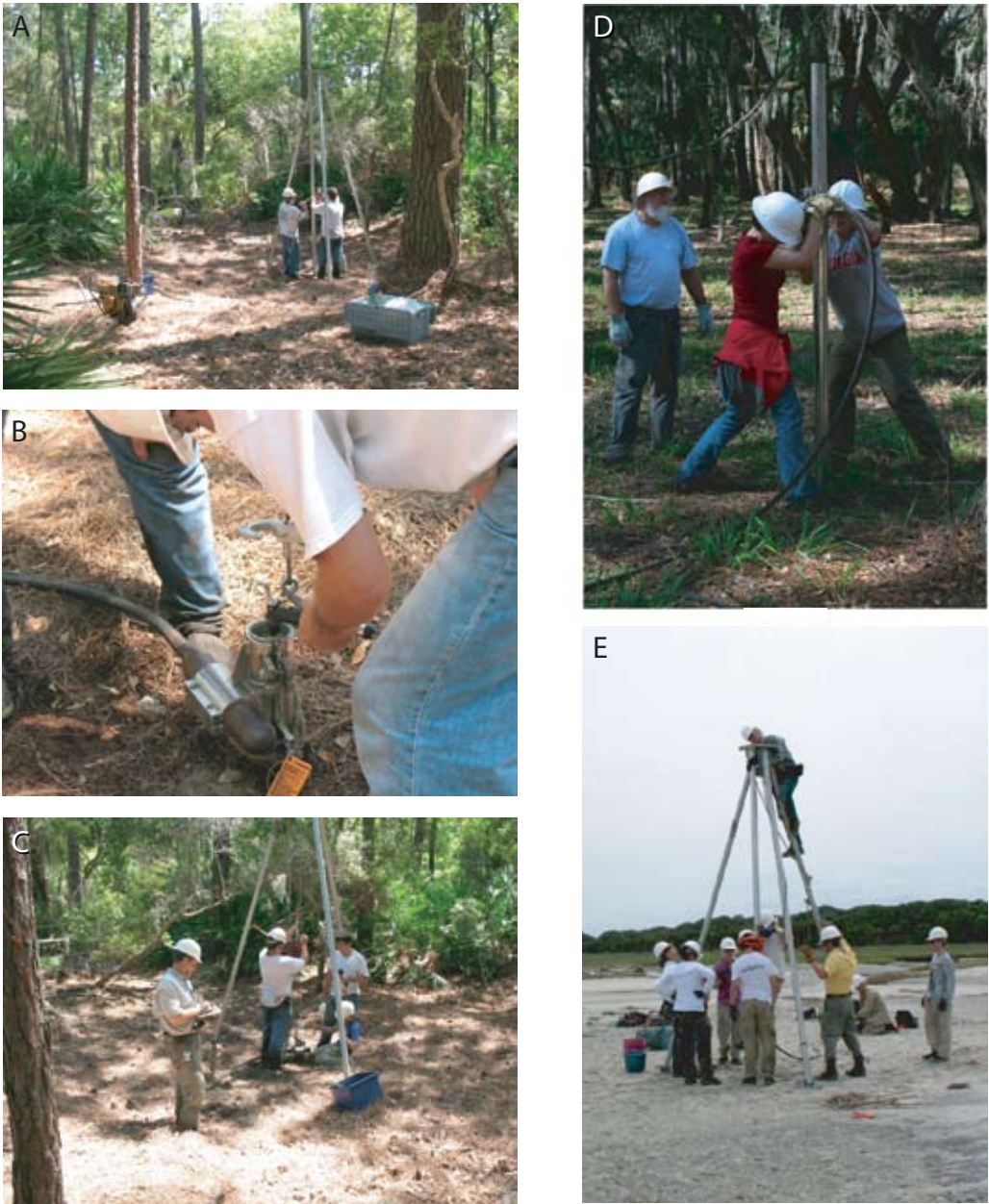
Fig. 10.1. Components of the St. Catherines vibracore in use in the field. A , Georgia Southern University drill team vibracoring near Gator Pond in 2008, showing gasoline engine, vibrator cable clamped to aluminum pipe under tripod as clamp is being raised to continue drilling; B , close-up of vibrator head clamped to irrigation pipe at total depth as sewer plug is being inflated to seal core in pipe; C , core being extracted by come-a-longs as crew chief Vance records data; D , AMNH crew coring at St. Catherines Shell Ring as crew chief Bishop supervises forcing the pipe into dry ground; E , Island Ecology Program coring at Flag Lagoon supervised by crew chiefs Potter (on tripod) and Keith-Lucas (kneeling) attempting to pull a core. Photographs A, B, C, and E by Gale Bishop; D by Anna Semon.
