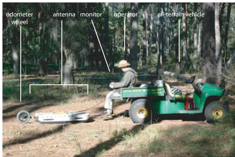
Fig. 11.2. GPR reflection profiling system used on St. Catherines Island to obtain over 20 km of profiles along the island road network. This MALA GPR system includes a 100 MHz antenna with attached control box and odometer wheel towed by a John Deere Gator ATV. Operator (R.K. Vance) sits with monitor and battery pack in a shoulder-mounted harness linked to control box by serial cable and power line (photograph by Lisa Vance).
