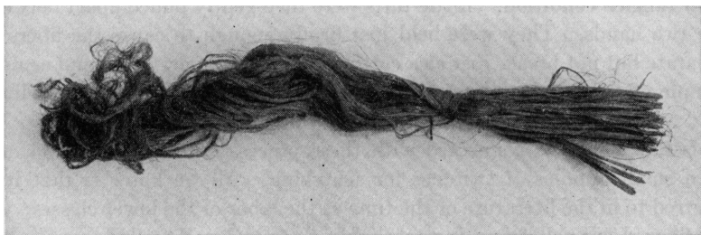
Fig. 8 (B-3472). Bundle of partially heckled Maguey Fiber. Length, 49 cm.
