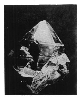
Fig. 1. A selectively coated quartz crystal. The faces of  $(10\overline{1}1)$  have included during the last stages of growth of the crystal an amount of colloidal clay substance, while the faces of  $(01\overline{1}1)$  and  $(10\overline{1}0)$  are not coated and present the ordinary transparent quartz of the crystal. The clay charged zone is cream white in color and is about 1 mm. thick. Alexander County, North Carolina.  $\times 1/2$
