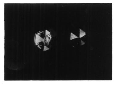
Fig. 2. Quartz crystals exhibiting a selective coating of the faces of  $(10\overline{1}1)$ ; the three alternating faces of  $(01\overline{1}1)$  are not coated. The crystals are viewed along the c-axis. La Grange, Troup County, Georgia.  $\times 3$
