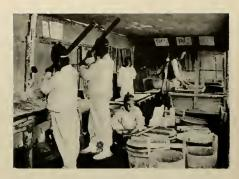
MACERATING MATERIAL IN KOREA. Age-old principles are used in modern paper mills, but only in the Orient is the work done extensively by hand
