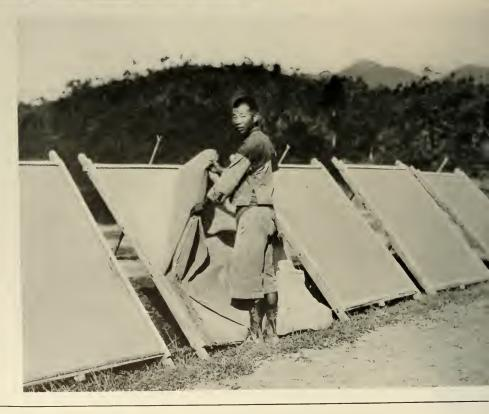
REMOVING THE PAPER AFTER DRYING: an ancient process widely used today. Unlike the cloth moulds shown in the upper picture, these are woven of rattan and leave a wicker-work impression on every sheet of paper
