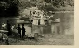
Bridgeless rivers like the Loya near Angumu are crossed on primitive ferries. Several boats are fastened together to support the car and are pulled along a cable
