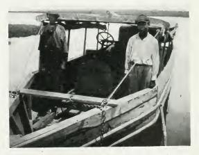
The "Creation," a homemade motor-boat used for towing barges of sugar cane. The motive power is a topless and wheelless Ford car
