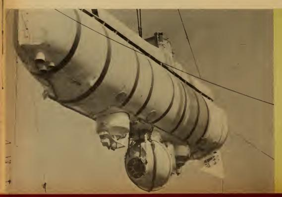
In 1960, the U.S. Navy's bathyscaphe *Trieste*, a special deepdiving submarine, carried two men in its ball-shaped cabin to the bottom of the Challenger Deep in the Pacific Ocean. It rested on the bottom, 35,800 feet down, for 20 minutes in the deepest dive man has ever made.
