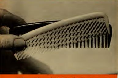
2. Two similar combs held together, but at an angle, produce an interesting moiré pattern. The wavy lines show that the comb teeth are not exactly evenly spaced. Scientists use moiré patterns to find flaws in materials.
