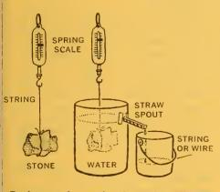
Equipment for testing loss of weight of an object immersed in a liquid. You can use paper or plastic containers and half of a large soda straw for the spout. Cut \(^4\)-inch slits in one end of straw, spread flaps inside hole, and fasten flaps to wall with sticky tape. Drip candle wax around outside of hole to seal spout.
