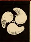
A boat propeller is called a screw. It "lifts" the water from in front of it to a position behind it, thus moving the boat.
