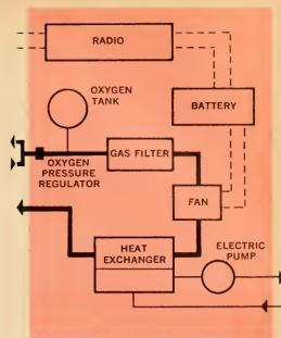
The back pack gives the astronaut the oxygen and air pressure he needs for life. Without it, he would die in an instant. This diagram shows what is inside the back pack and how it works.
