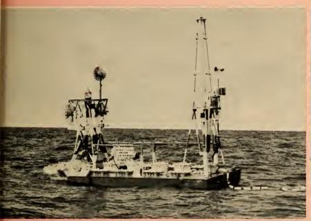
NOMAD I weather station is one of many automatic stations that makes observations in remote parts of the world. This one, designed by the Navy to operate at sea, measures wind direction and speed, air pressure, air and water temperature, and has a trial attachment for measuring solar radiation. NOMAD I radios its findings to a nearby land weather station.
