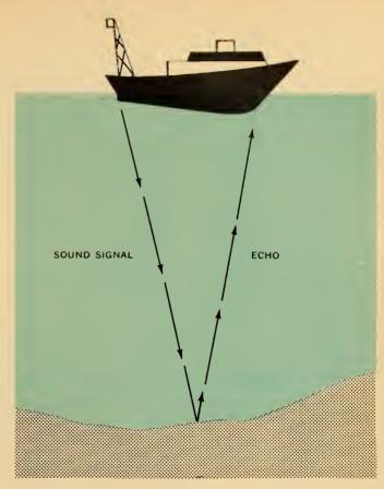
The echo-sounder is an instrument that sends out sound signals in the form of "pings," one every second or so. The length of time it takes a ping to reach the sea bottom and then bounce back to the ship as an echo tells scientists exactly how deep the water is beneath the ship. As the ship moves along, the echo-sounder draws a continuous line on a moving piece of paper. The line shows the profile, or shape, of the sea bottom.
