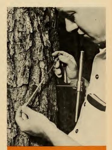
Foresters use a device called an increment borer to see how fast a living tree is growing. As the borer is twisted into a tree, it cuts a rod-like core of wood. This core can then be pulled out and studied. The core shown above has close-spaced annual rings near the bark, a sign of slow growth in recent years.
