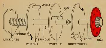
wheels turn freely around the *spindle*. One end of the spindle fits into the end of the shaft, the other end is attached to the loek ease. (The shaft and spindle may be arranged differently in some kinds of loeks.)
