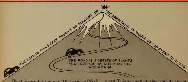
The staircase, the ramp, and the road up Pike's Peak are all *inclined planes*, or surfaces that slant. To lift yourself—or a piano—upward on an inclined plane, you also have to move for-
