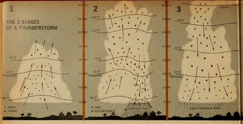
These diagrams show the three stages of a growing thunderstorm: 1. In the cumulus stage the cloud has updrafts only. Rain droplets are not heavy enough to fall out of the cloud. 2. In the mature stage there are downdrafts as well, which Inside a Thunderstorm (continued)
