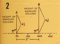
Vertical line A represents the height of the mercury column in a gas thermometer when the gas is at the melting point of ice (0°C); vertical line B, the height of the mercury when the gas is at the boiling point of water (100°C). For each degree of temperature rise or drop, remember, the mercury rises or drops by the same amount.
