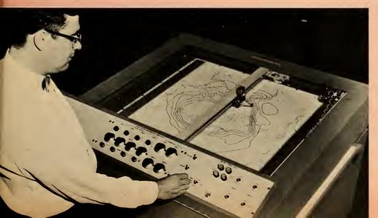
Wiggly lines (called isobars) are being drawn on this weather map of the Northern Hemisphere by a computer. After information about air pressure from weather stations around the world has been fed into the computer, and sorted out by the machine, the computer draws the map in three minutes. Drawing it by hand takes more than an hour.
