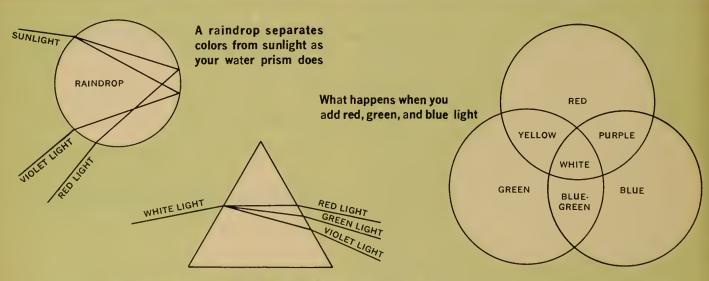
Light of shorter wave lengths bends more than light of longer wave lengths when passing through a prism
