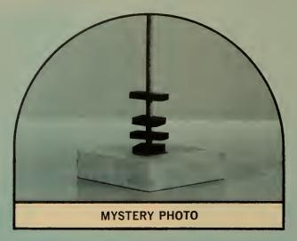
The photograph shows some ring magnets with a stick running loosely through the holes in the magnets. What do you notice about the spaces between the different magnets? What causes this?
