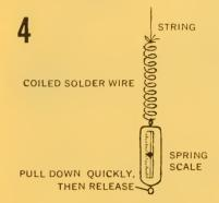
Take two lengths of solder wire, each 2 feet long, and coil each of them around a test tube or other cylinder about the same diameter. Wind the coils as close together as possible.
