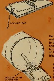
Tape an extension (about  $1\frac{1}{2}$  or 2 inches long) onto the trigger of a mouse trap. You might use a popsicle stick.
