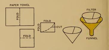
To make a filter, fold a sheet of paper towel twice, then cut off the unfolded corner, as shown above. Open the paper to form a cone and place it in the kitchen funnel.
