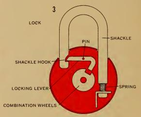
middle, pushing the other end of the lever into the slots in the edges of the wheels. This releases the hook so that the end of the shackle can come out of the lock.
