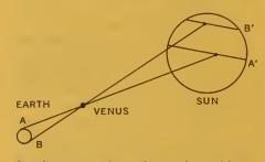
An observer at A on the earth would see Venus cross the sun's disc along path A' during transit. An observer at B would see the planet cross at B'.
