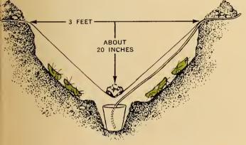
This scientist is drawing water into a collecting jar to measure the amount of drinking water produced by his plastic-sheet-and-bucket solar still set up in the desert. The sheet of plastic hangs into a hole about 3 feet across. A rock keeps the tip of the plastic cone above the bucket. Water vapor from the ground, and from chopped-up plants, condenses on the plastic and drips into the bucket.
