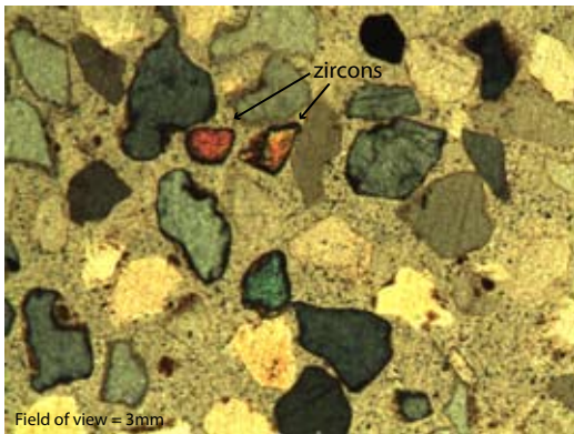
Fig. 4.10. Photomicrograph of 5A horizon under cross-polarized light at 50x. Note zircons in photo (high birefringence grain) and strong angularity of the fine sand-sized quartz grains. Also note abundant disseminated organics. Photomicrograph taken by Frank Vento.
